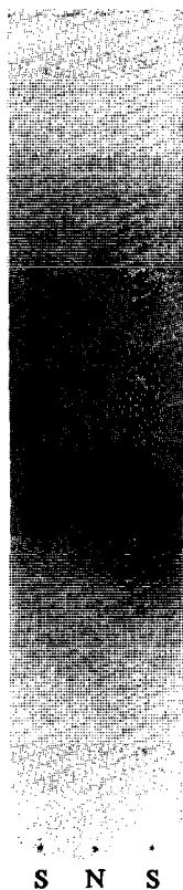
FIG. 3. Thin-layer chromatogram of natural (N) and synthetic (S) malformin A_1 , on silica gel with water-saturated ethyl acetate as solvent.
